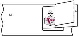
9. Remove any bubbles by using the corner of a razor blade or a sharp pin or needle and a rolling thumb.
